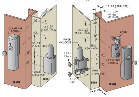
**NOTES:** Either **F** Dimension or **G** dimension must be less than 19.8 (.78) for the door to open a full  $180^{\circ}$ . # Dimension will vary as  $\dagger$  dimension is adjusted through its range. The door and frame design must allow for this variation.
