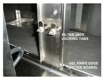
STEP #1 - TURN ALL FILTER JACK TABS PARALLEL TO FILTER KNIFE EDGE ON UNIT TO ACCOMMODATE FILTER
